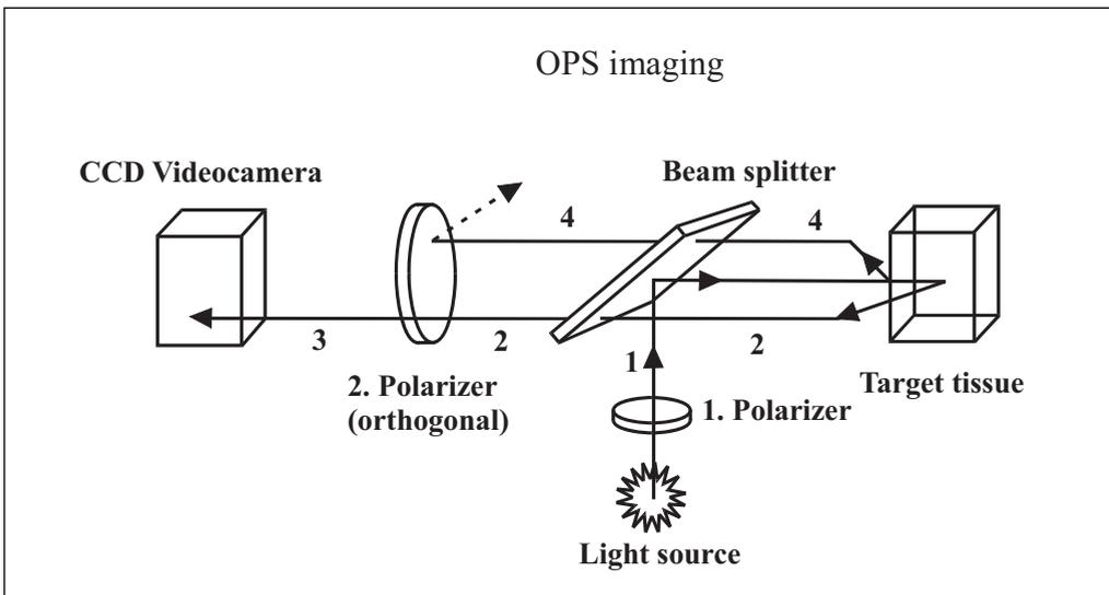
Figure 2: OPS imaging, optical scheme. (1) Incident polarized light is reflected toward the target tissue by beam splitter (2). Depolarized scattered light passes through orthogonal polarizer-analyzer and (3) it is projected onto CCD videocamera. (4) Reflected polarized light eliminated by orthogonal polarizer (adapted from Cerny, 2006)
